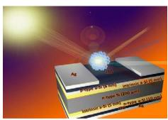
Introducing the next generation of solar cells! They are silicon solar cells with graphene flakes incorporated into them expanding the usable light range in silicon solar cells to improve their efficiency. Also read this <u>ACS</u> article for additional information.
